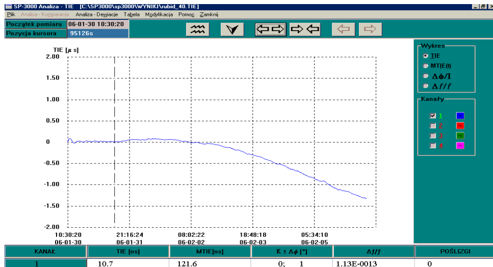
Fig. 4. Exemplary diagram of the Time Interval Error TIE of the LPFRS generator for the ambient temperature of 40°C in non-synchronized mode.
